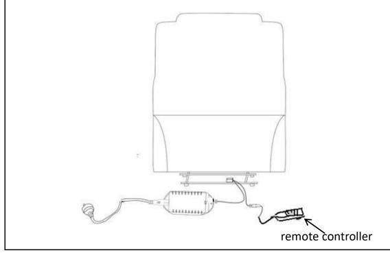
Back-up Power Option: This electric lift chair has been equipped with a Safety Battery Back-up Option. This battery back-up function is important to use when the electricity supply stops (power outage). Please ensure you place 2 X 9 volt batteries into the transformer piece during assembly.
